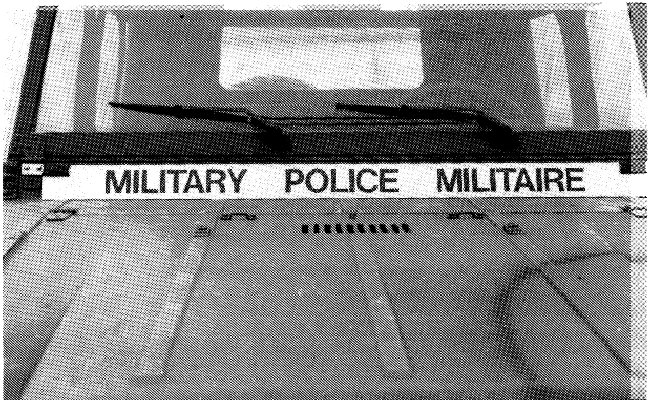
Figure 15 Installation of Front Sign Under Windshield
