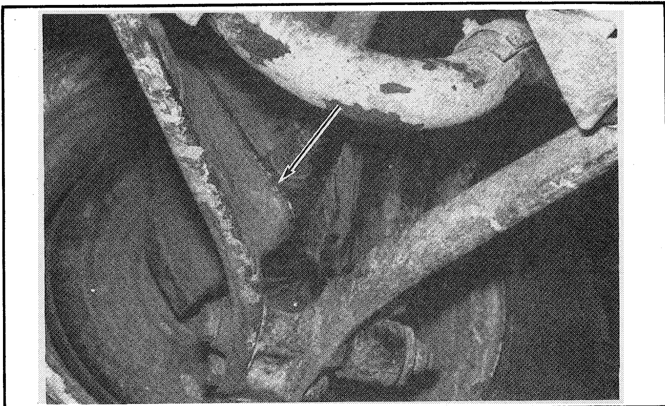
Figure 2 Guard Installed Inside Wishbone
