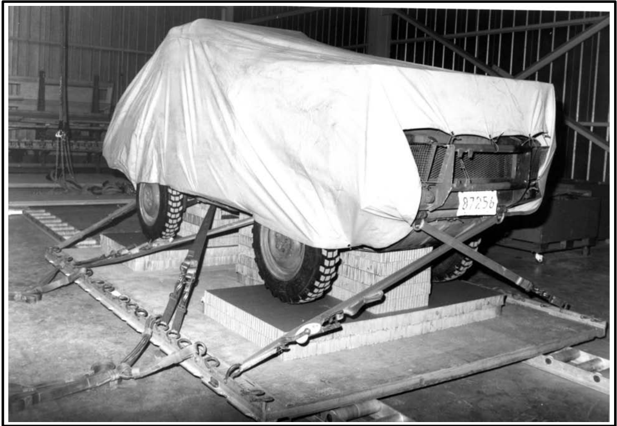
Figure 2-7 Canvas Cover Installed
