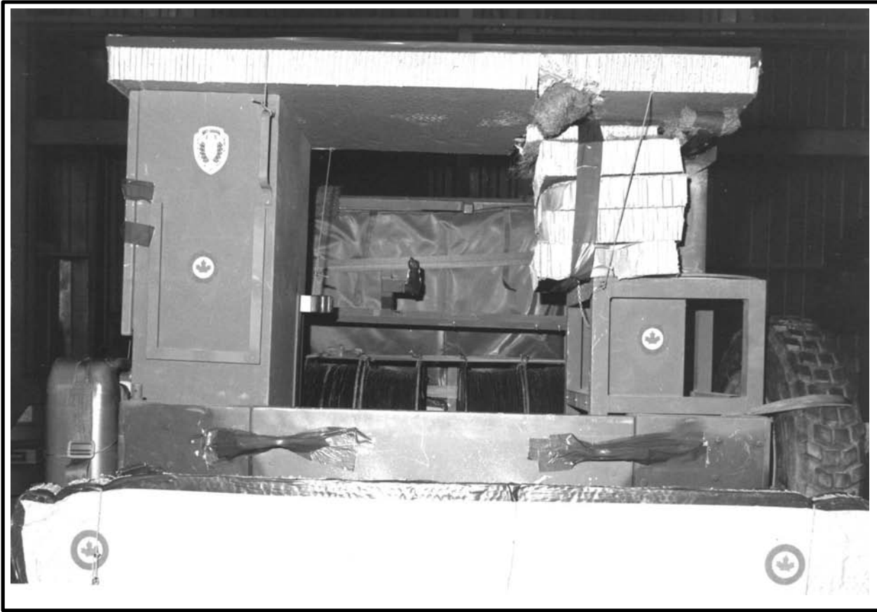
Figure 6-24 Reeling Machine Honeycomb Support and Honeycomb Plus 3/4-inch (6.35 mm) Plywood Across Top of Storage Container
