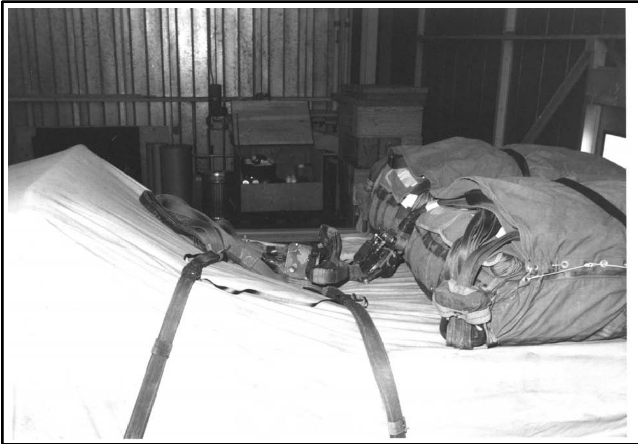
Figure 4-25 Suspension Slings Safe-tied
