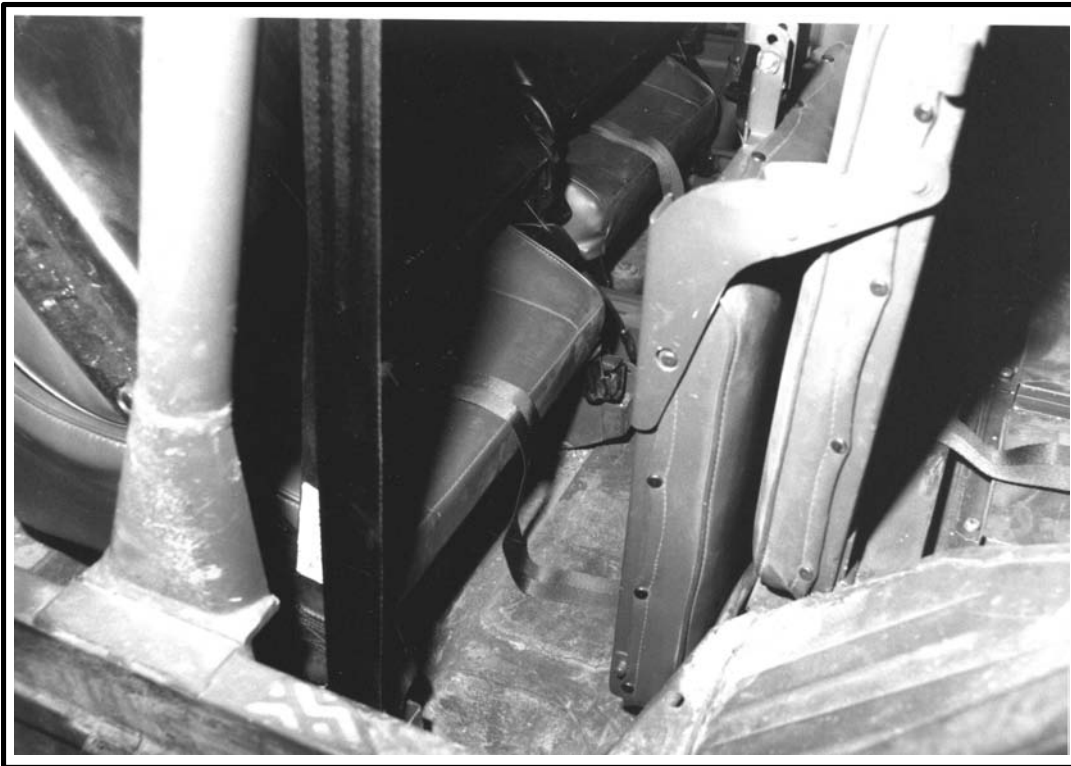
Figure 1-4 A7A Strap Routing Under Seats
