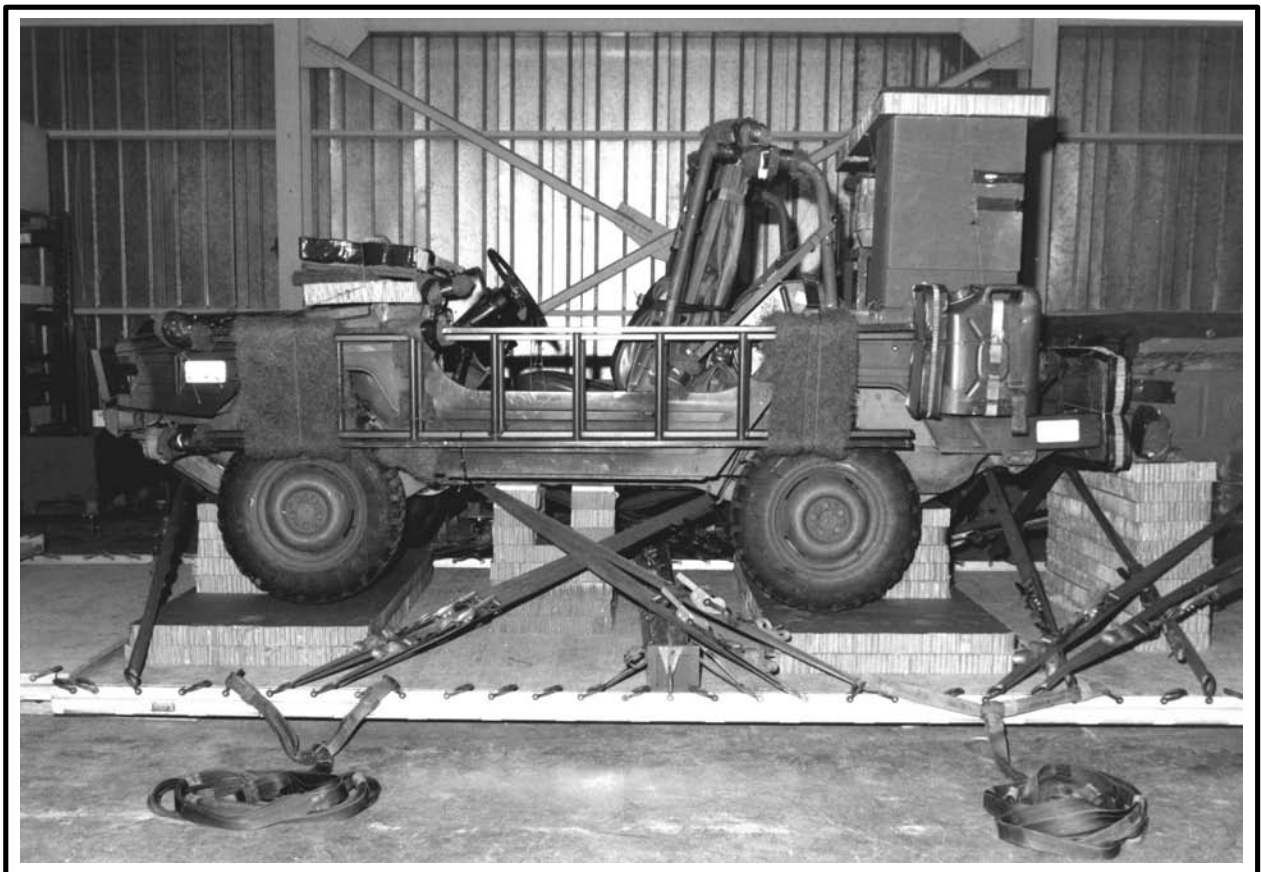
Figure 6-31 Poles Installed and Secured
