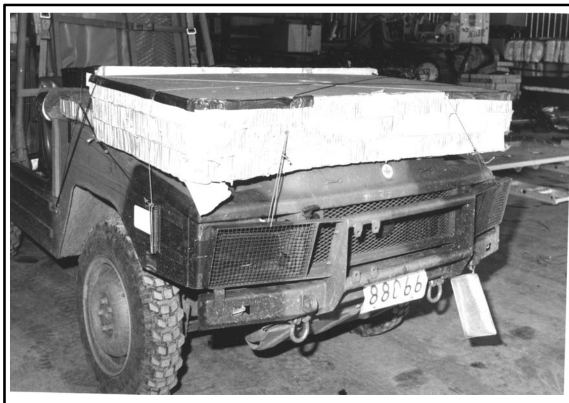
Figure 6-28 Parachute Tray Installed
