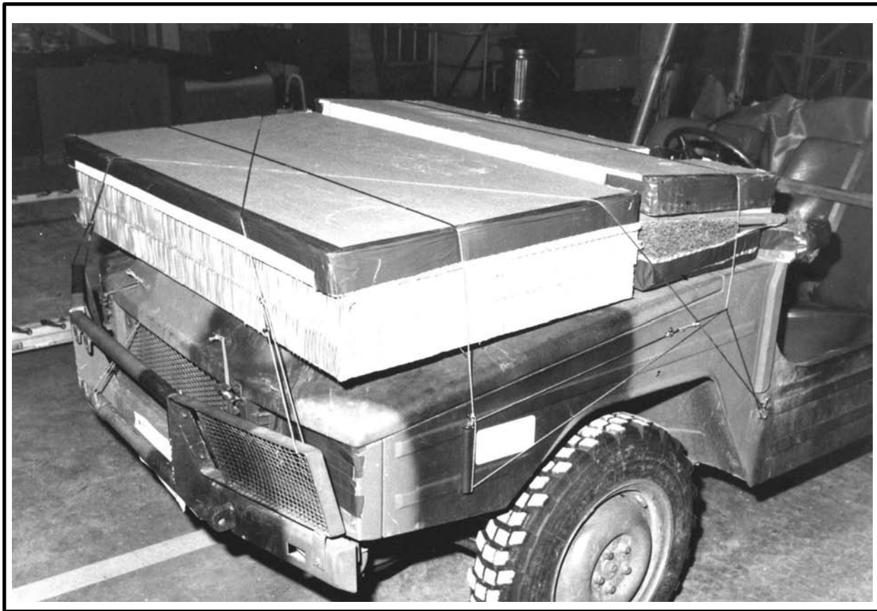
Figure 2-3 Parachute Tray Installed
