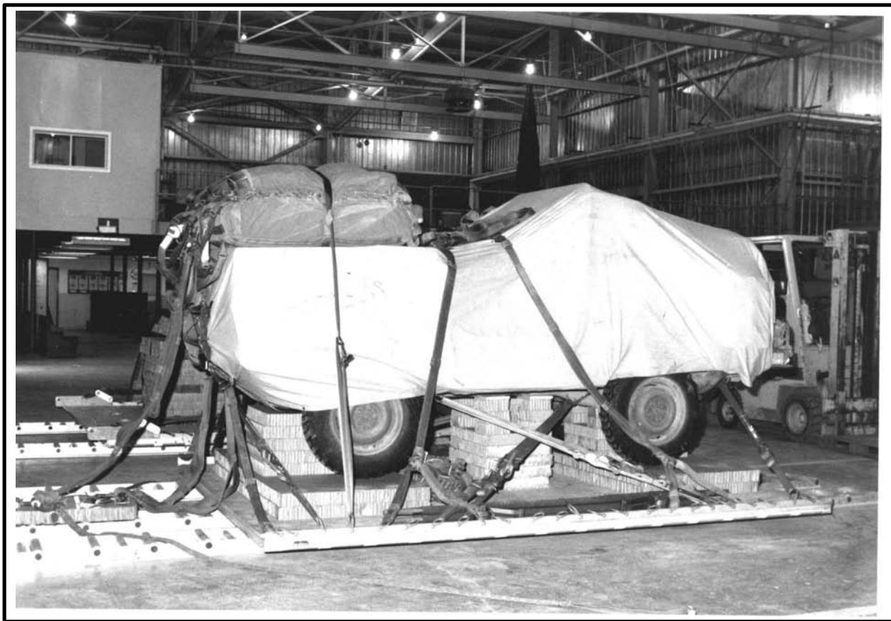
Figure 2-10 ILTIS rigged for LVAD
