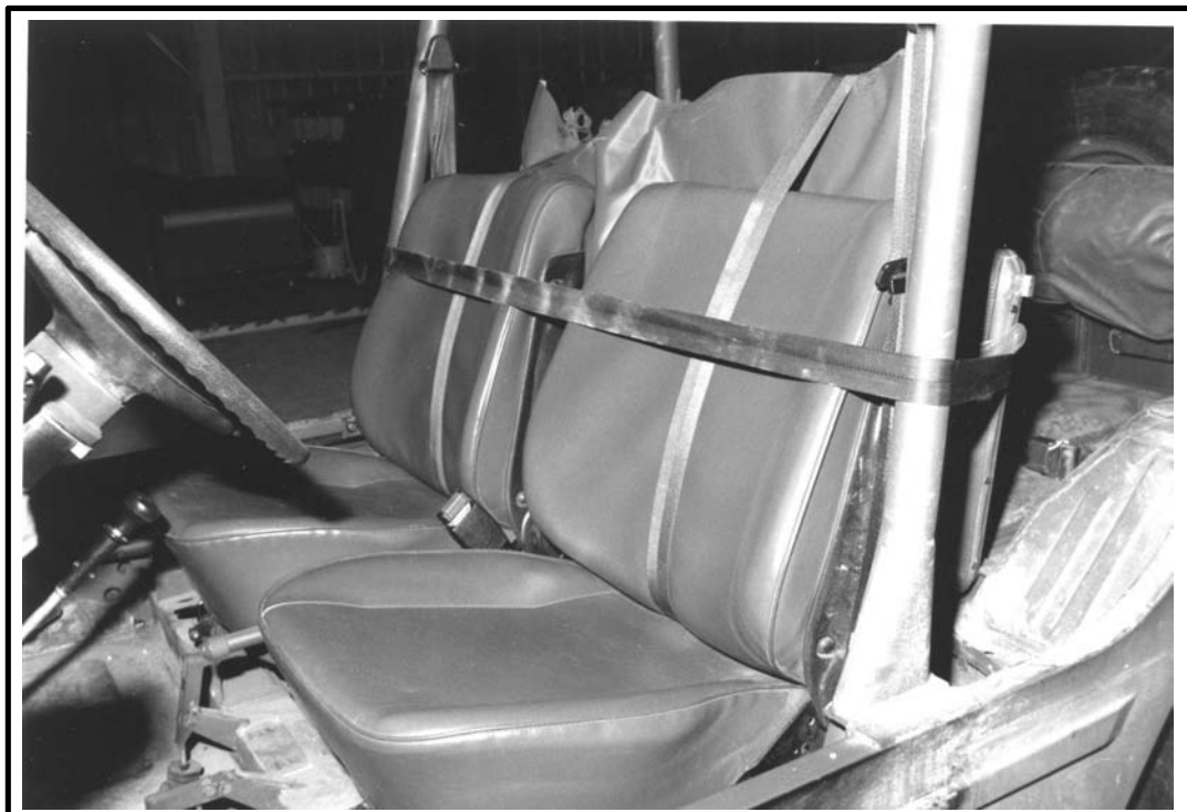
Figure 1-6 A7A Straps Installed (Front View)
