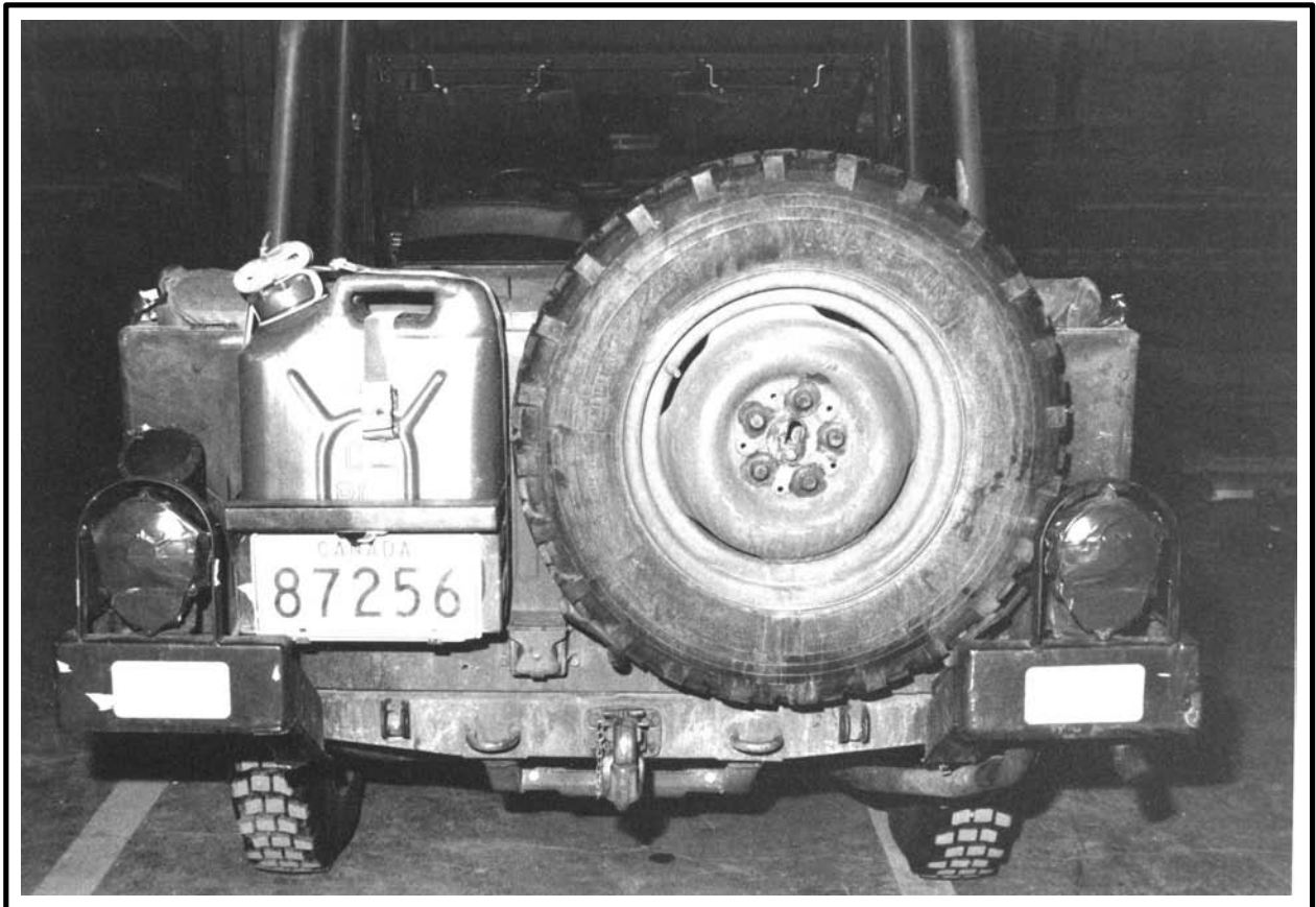
Figure 1-11 Gas Can and Spare Tire Secured
