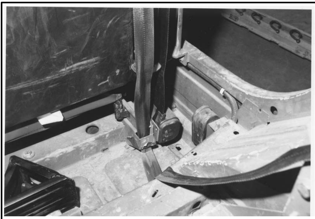
Figure 6-9 A7A Straps Through Outboard Seat Support Bracket
