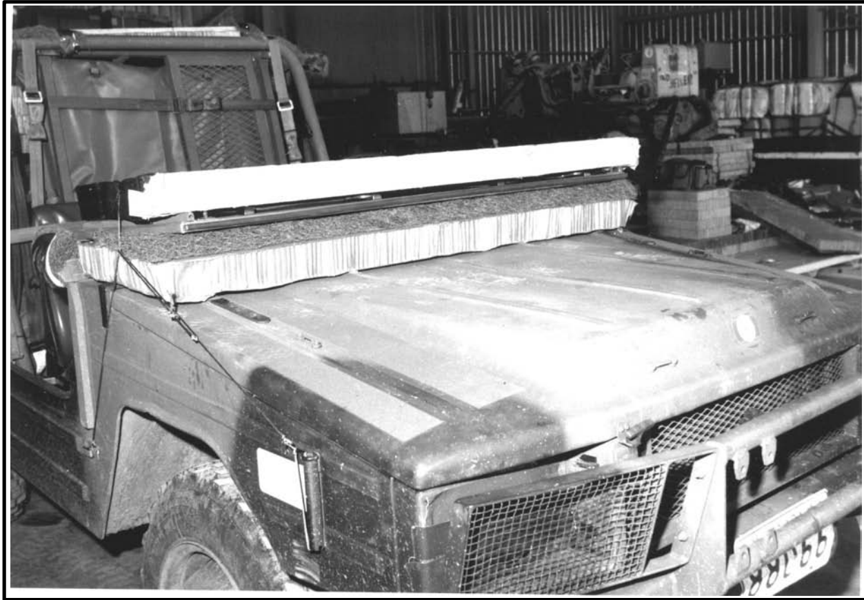
Figure 6-26 Windshield Protection Installed
