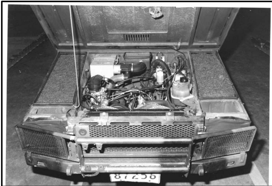
Figure 1-7 Tool Storage Wells – Excess Space Filled
