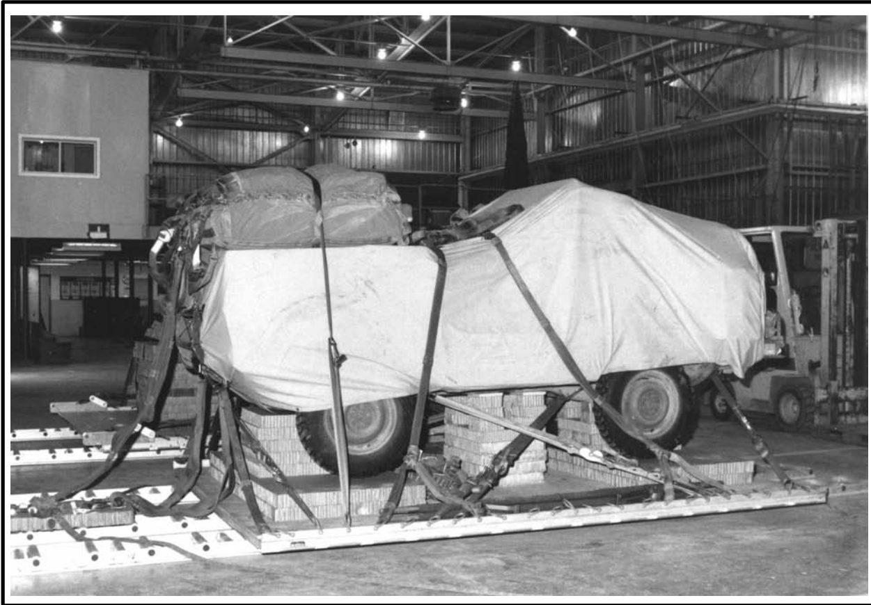
Figure 4-26 ILTIS rigged for LVAD
