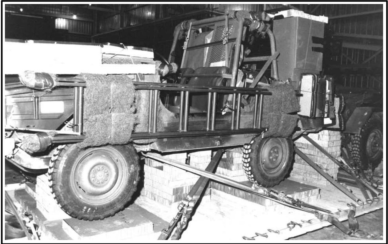
Figure 6-25 Ladder Secured in Position
