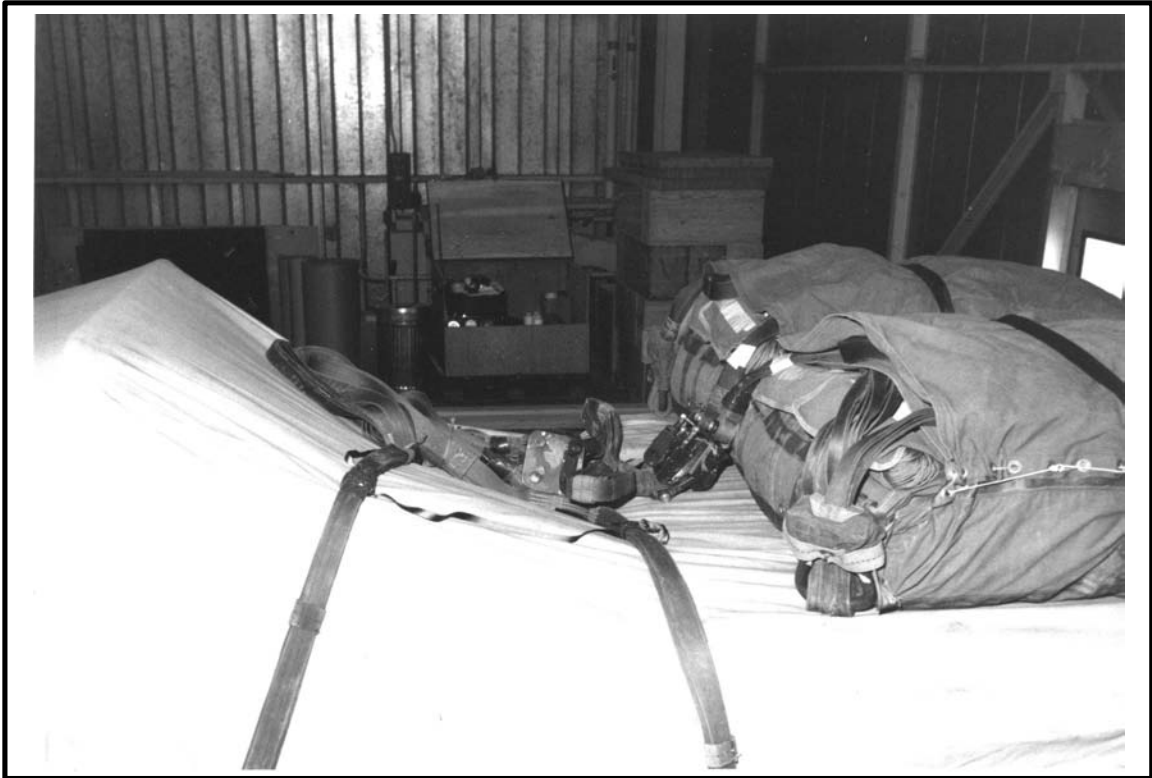
Figure 2-9 Suspension Slings Safe-tied
