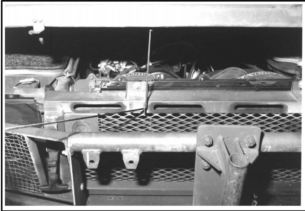
Figure 6-14 Type III Nylon Cord through the Locking Hole on Hood
