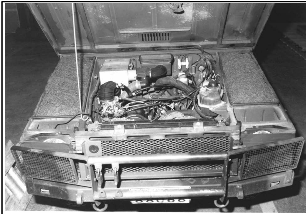
Figure 6-13 Tool Storage Wells Excess Space Filled with Horsehair
