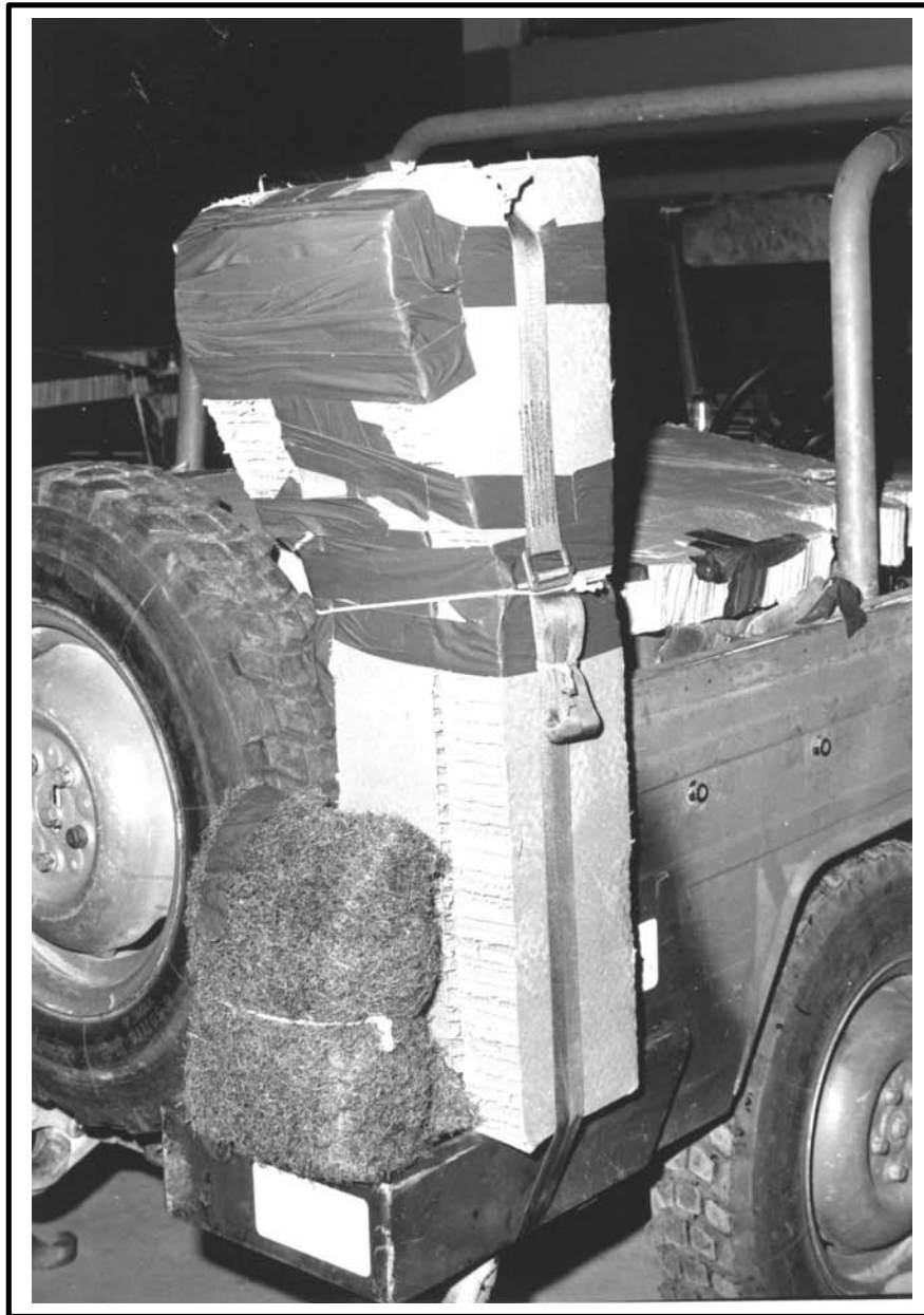
Figure 1-13 Antenna Mount Protection Installed and Secured Figure 1-13 Protection de support d'antenne installée et fixée
