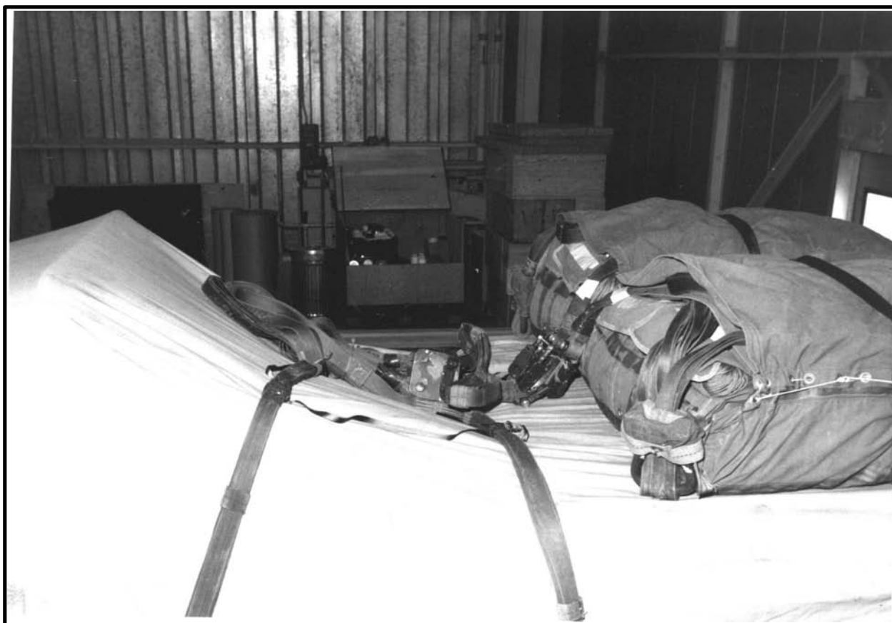
Figure 6-33 Suspension Slings Safe-tied
