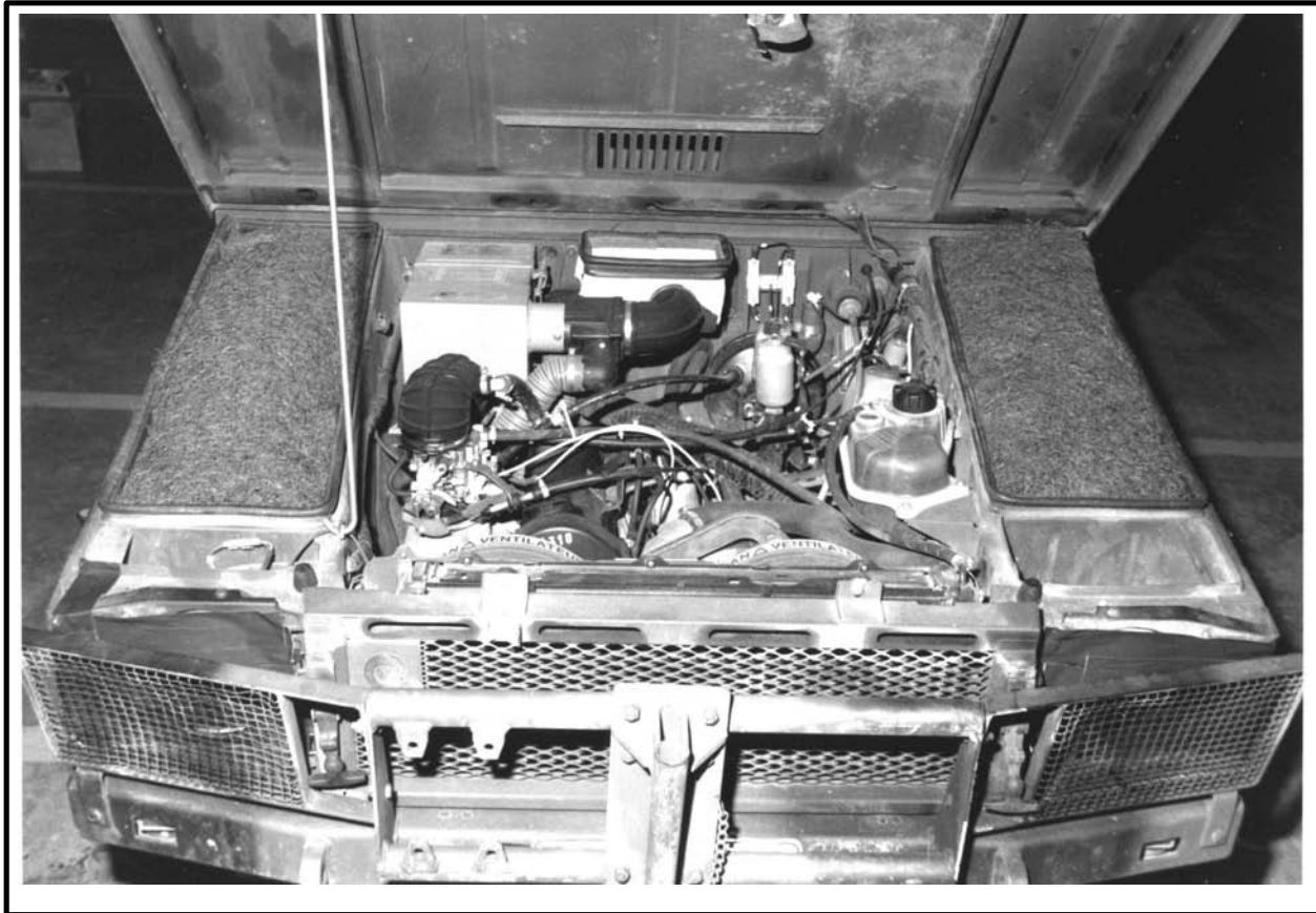
Figure 4-11 Tool Storage Wells Excess Space Filled with Horsehair
