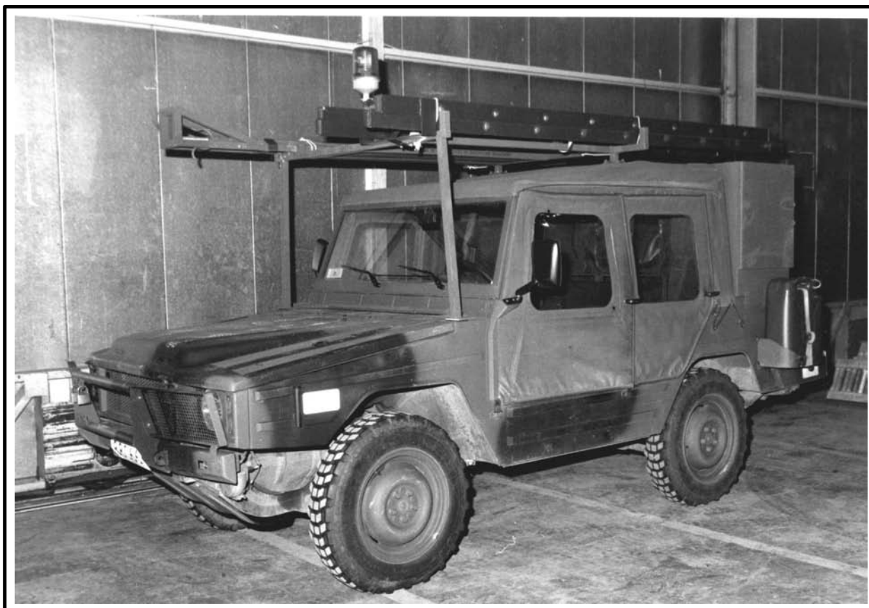
Figure 6-1 The ILTIS Cable Layer
