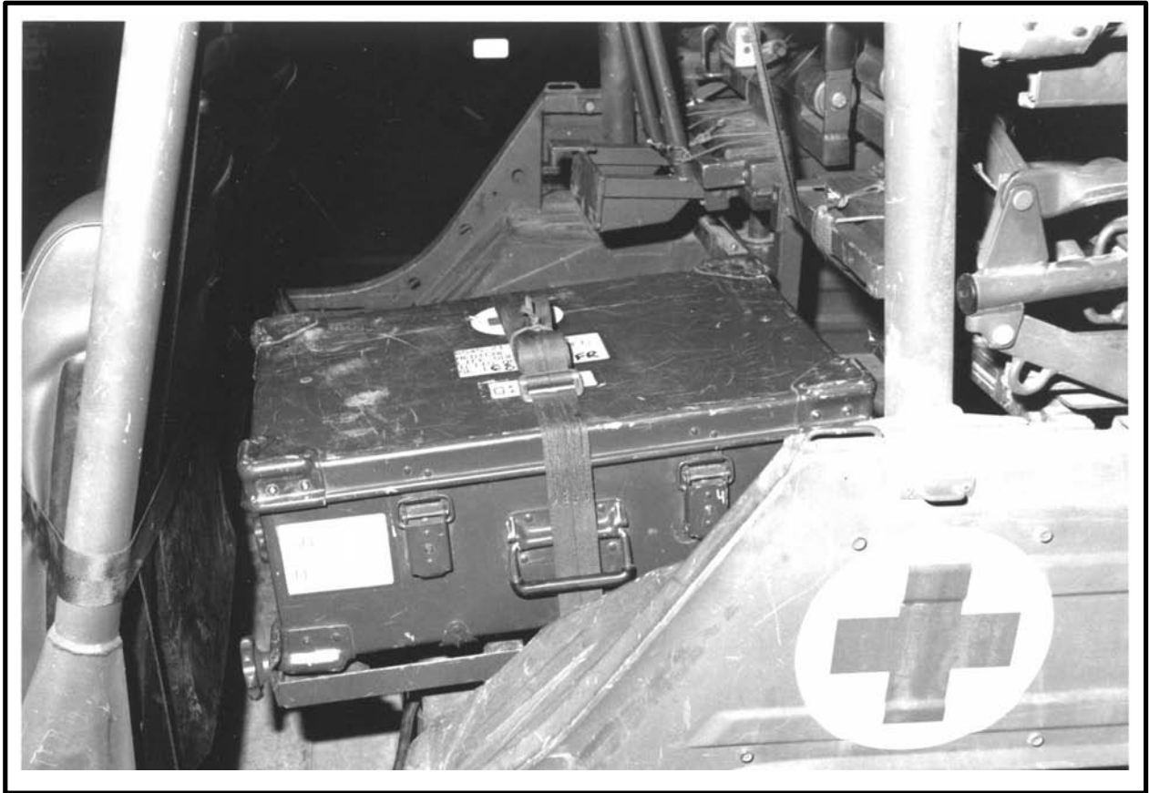
Figure 4-16 Medical Supply Box Secured
