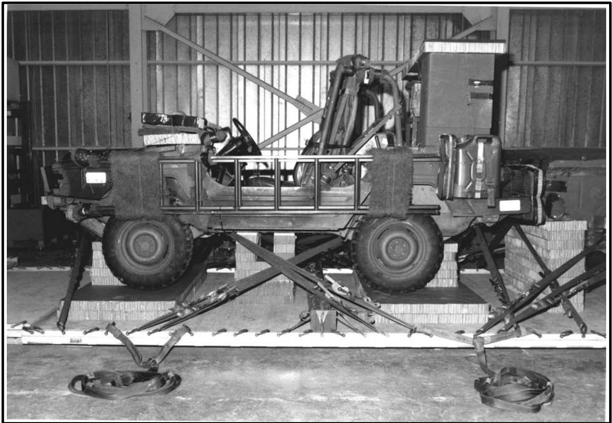
Figure 8-15 Poles Installed and Secured
