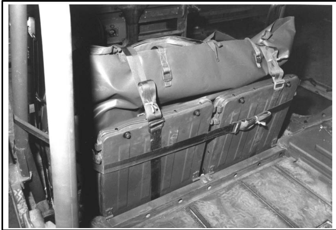
Figure 1-5 A7A Straps Installed (Rear View)
