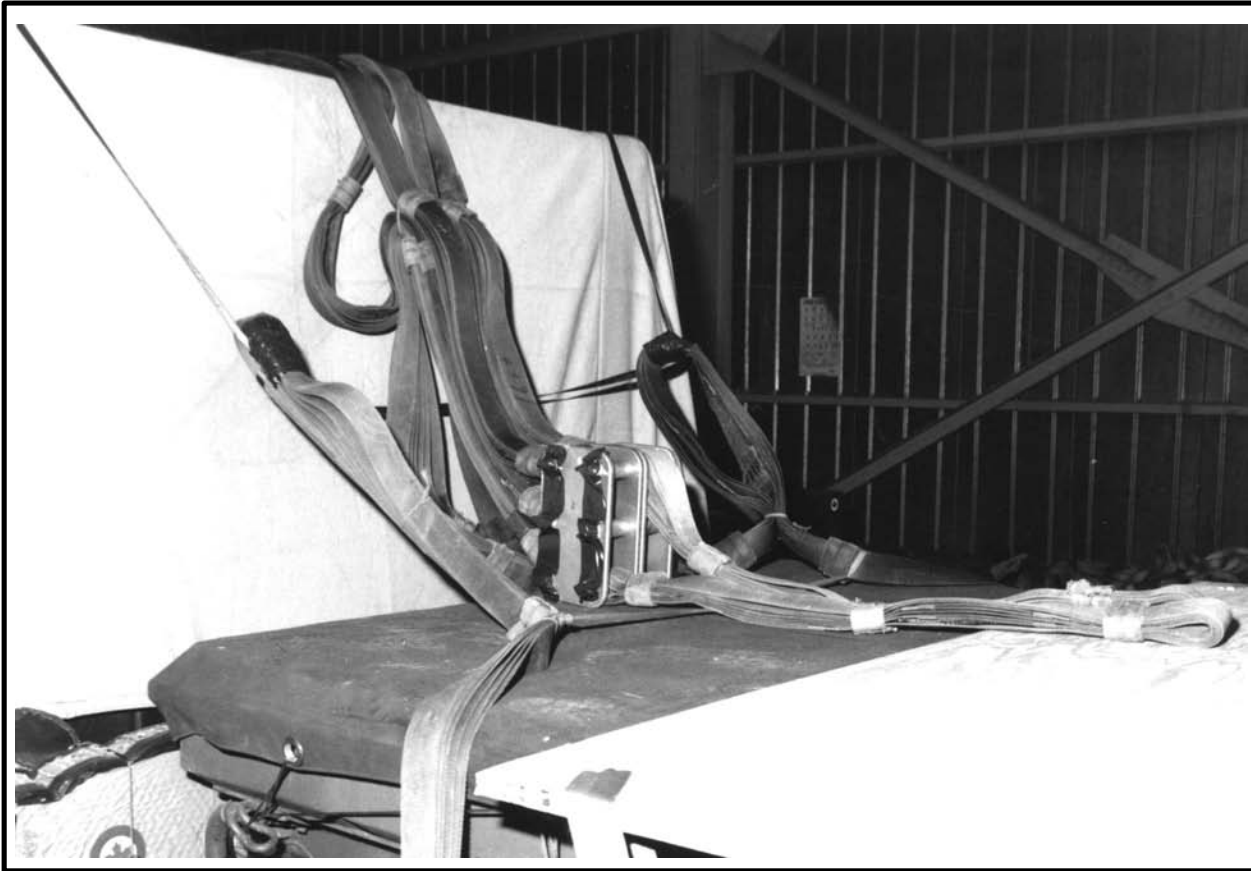
Figure 8-18 Suspension Slings Safe-tied
