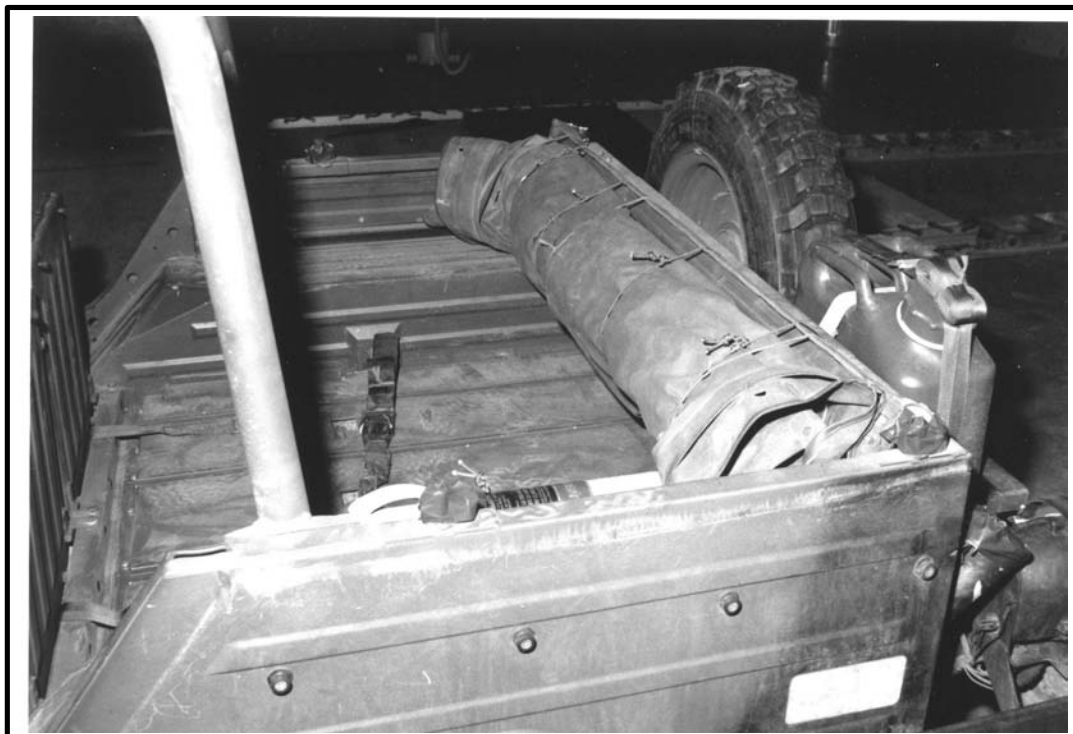
Figure 1-3 Rolled Tarp and Frame Secured
