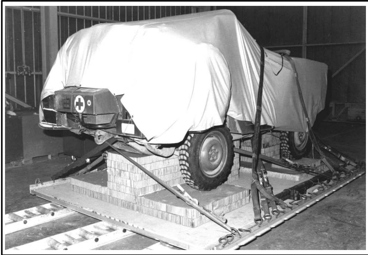
Figure 4-23 Installation of Canvas Cover
